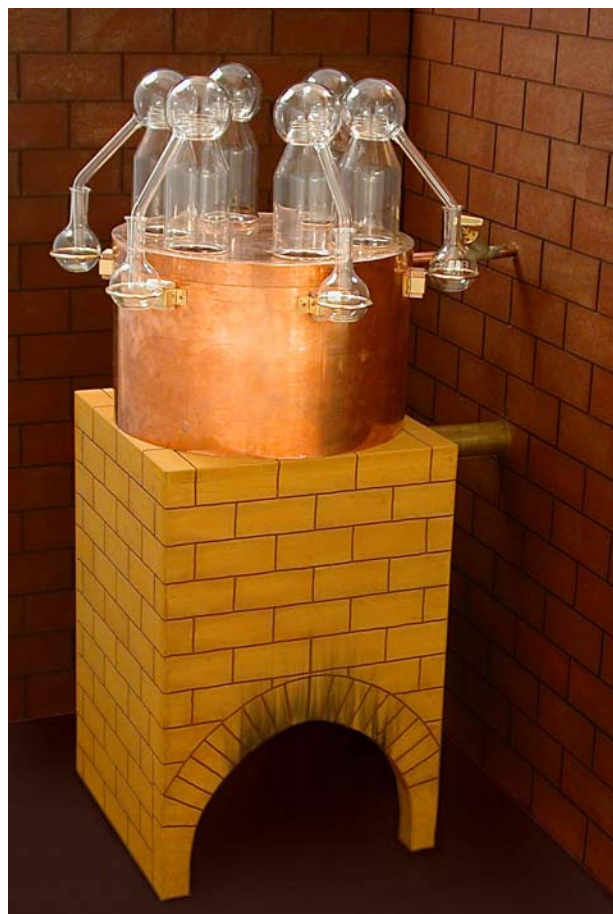
Our model: Copper and wood, laminated. 6 alembics of glass. Total height 1.2 m. (Inventory No. K 1.63)
