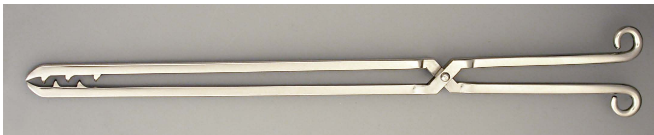
Model (a): Stainless steel, riveted. Length: 254 mm. (Inventory No. H 6.03)
