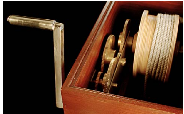
Our model: Wood and brass, Copper weight (8 kg) (Inventory No. E 1.12)
